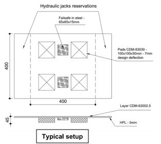
The acoustical consultant, defined a solution with elastomer bearings having a natural frequency of 8-10 Hz, because of the proximity of the railway track and an important car traffic road.
