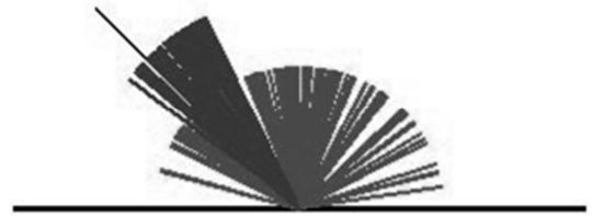
Fig. 5a: The Lambert directivity (cosine-function); 5b) reflected ray distributions simulated by drawing random numbers for scattering coefficients of 0, 0.25 and 1.
