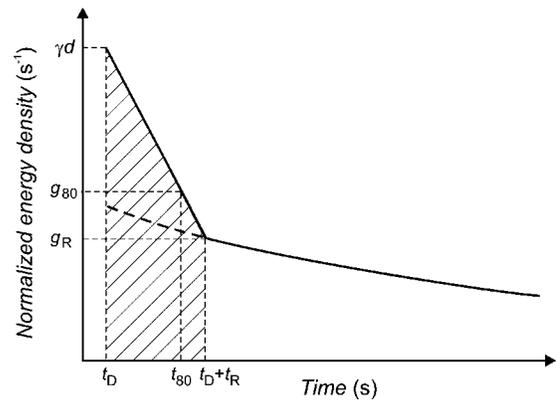
FIG. 1. Plot of the theoretical distribution of energy density of the reflected sound against the time according to the modified theory. The sound is emitted at time  $t=0$ , and reaches the receiver at  $t_D$ . From  $t_D$  to  $t_D + t_R$  the energy density follows a linear function, and then starts the purely exponential decay.
