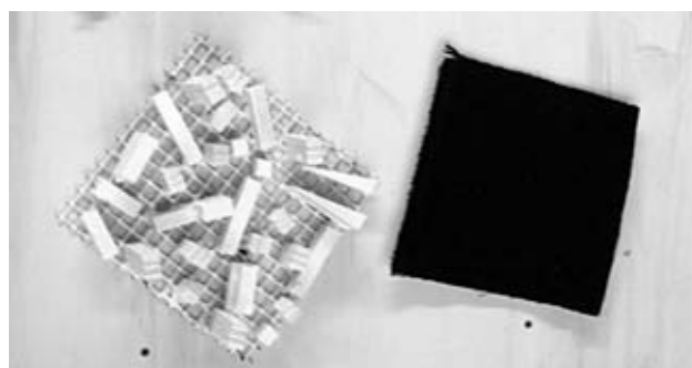
FIG. 2. The scattering (left) and absorbing (right) samples used in the setups of the model room.
