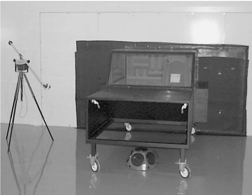
FIGURE 11.6. Photograph of a reverberation chamber. (Courtesy of Eckel Industries, Inc.)
