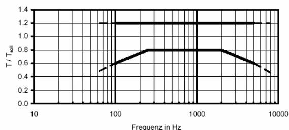
Figure 2 -DIN 18041:2004 tolerance band for the recommended reverberation time as function of the frequency: T reverberation time - T<sub>ot</sub> optimal recommended reverberation time of fig. 1.
