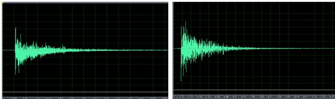
Figure 5.a -Simulate Impulse Response with software Odeon 6.0
