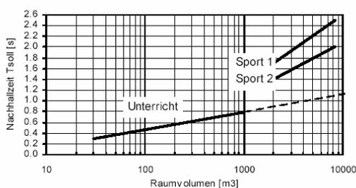
Figure 1-DIN18041:2004 optimal reverberation time, for the octave bands 500Hz and 1000 Hz, in function of the occupied room volume.
