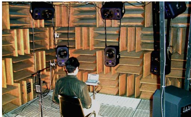
Figure 13. Photograph of the loudspeakers of the room acoustics simulator in the anechoic room.
